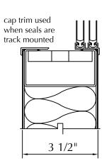
40 N.I.C. GUARANTEED WHEN SPECIFIED TESTED IN ACCORDANCE WITH ASTM E336
